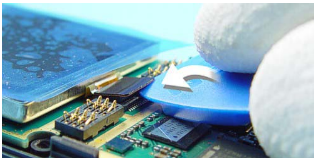
Use SRT-6 to open the LCD connector. Take care about components on the Engine Module during this procedure.
