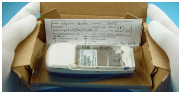
Add repair documentation e.g. filled-in service note into the swap carton.
