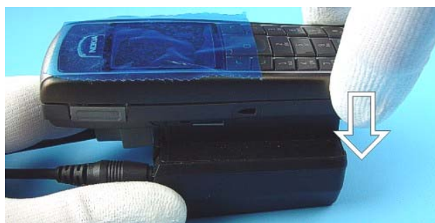
Now, push down the bottom side of the phone, do not use too much force.
