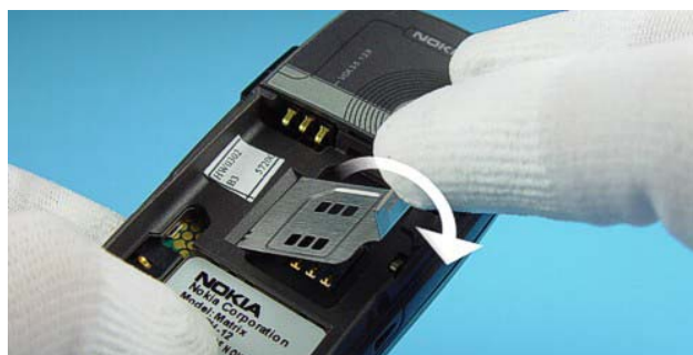
Close SIM Lid before inserting the Flash Adapter.
