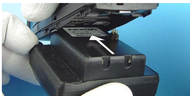
Insert the Flash Adapter SF-7 like a battery, start at the Battery Connector side.
